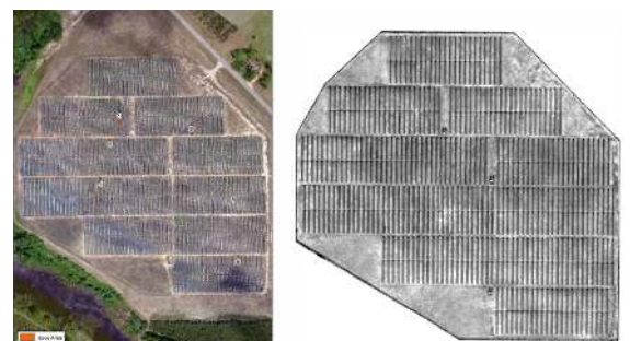
Figure 3.2 Malfunctioning Module Review. Visual orthomosaic displaying the issue areas containing malfunctioning modules (left.) Thermal orthomosaics are referenced for automatic malfunctioning module identification (right)..
